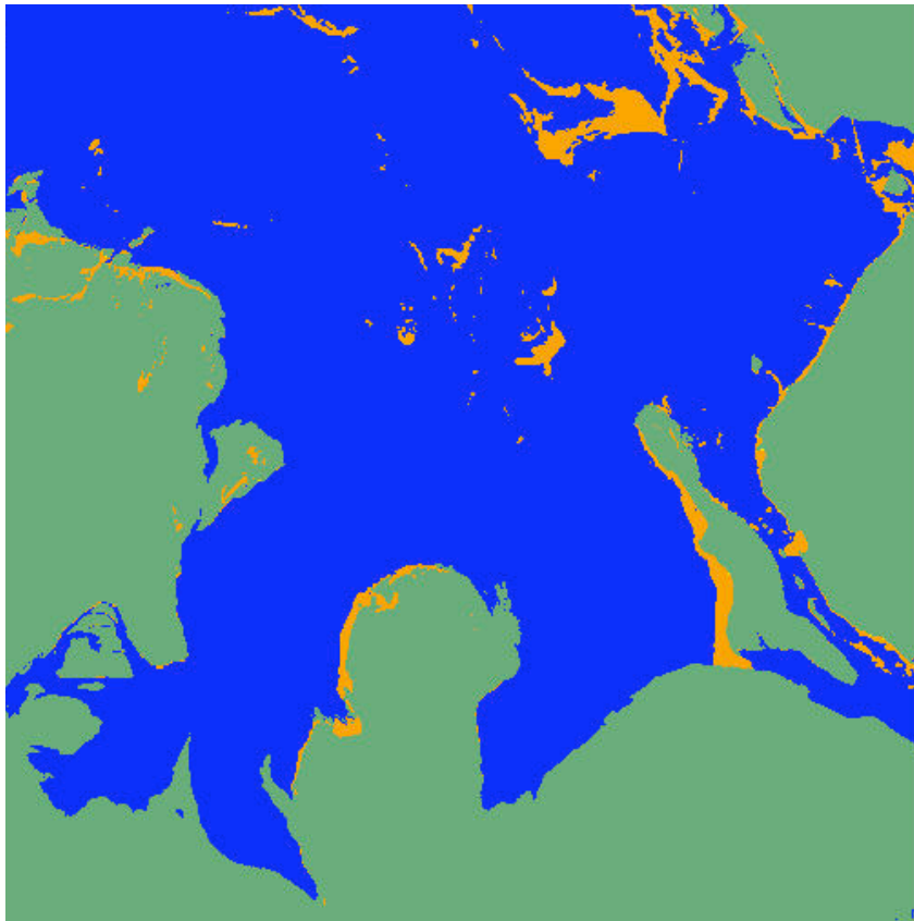
Figure 4. A Masked Pseudo-color density slice of the product of the values of TM Band 4 and TM Band 5.
